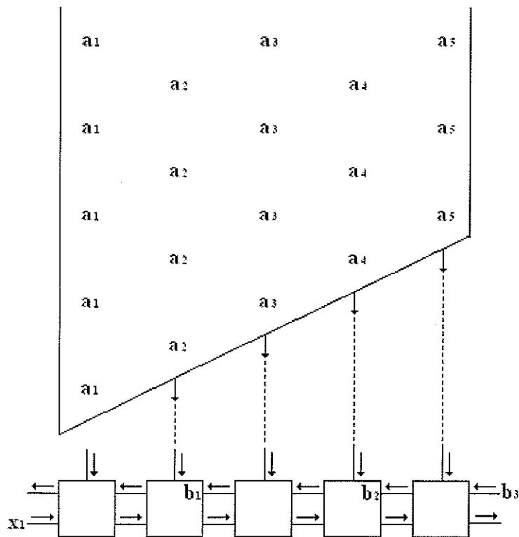
The first 9 steps of the convolution of vectors  $a$  and  $x$ .
